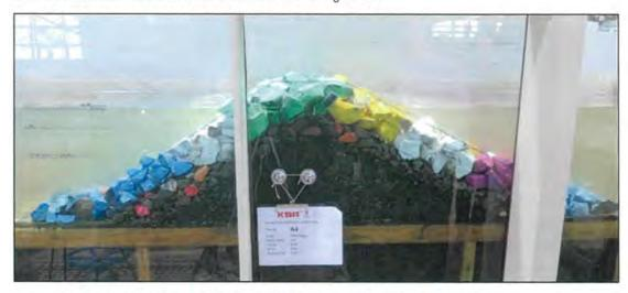
Figure 6.1 Concept physical model testing - Model cross-section (Test sequence A4)
