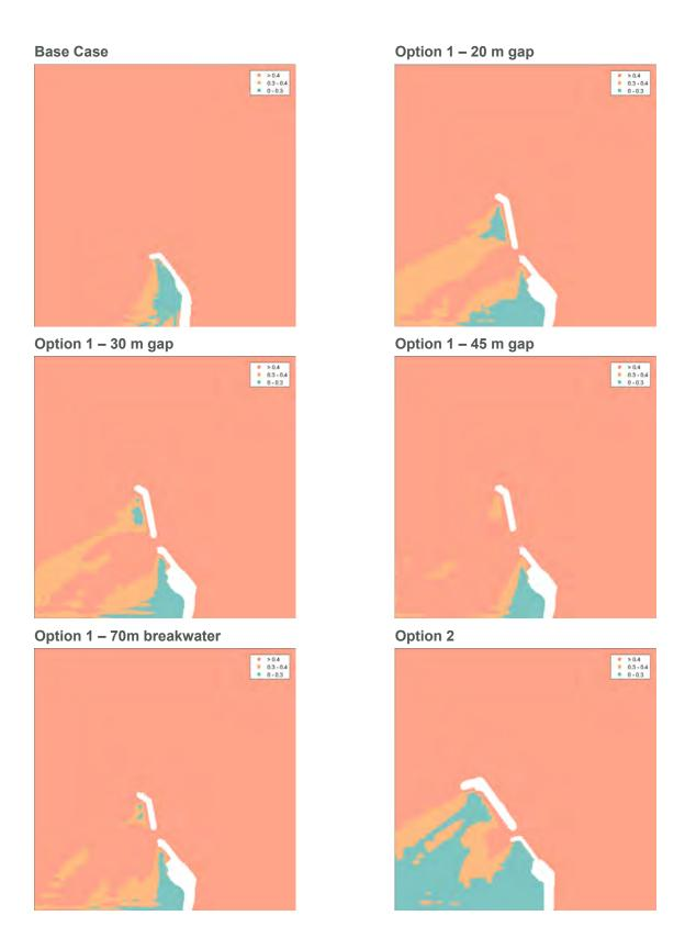
Figure 4-11 Significant wave height exceedance envelopes for 1 year ARI waves (all directions)
