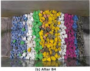
Figure 5.1: Overview of Tested Breakwater During Test Series B (left = leeward; right = offshore)
